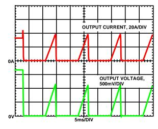
FIGURE 12. OVERCURRENT BEHAVIOR IN HICCUP MODE
