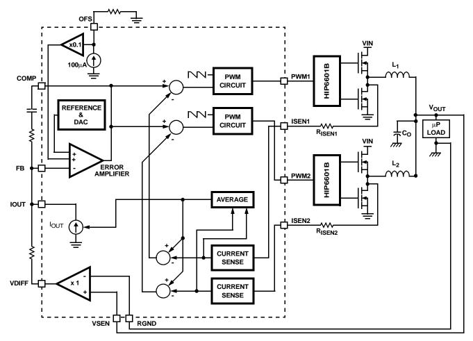
FIGURE 1. SIMPLIFIED BLOCK DIAGRAM OF A ISL6569A CONVERTER
