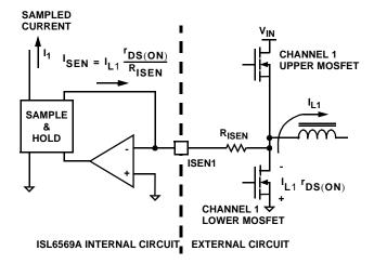
FIGURE 4. CHANNEL 1 INTERNAL AND EXTERNAL CURRENT-SENSING CIRCUITRY
