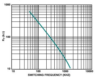
FIGURE 15. RT VS SWITCHING FREQUENCY
