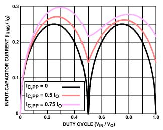
FIGURE 16. NORMALIZED INPUT-CAPACITOR RMS
