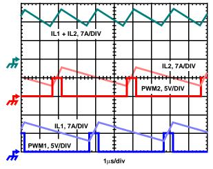
FIGURE 2. PWM AND INDUCTOR-CURRENT WAVEFORMS FOR 2-PHASE CONVERTER
