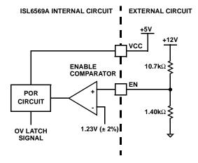
FIGURE 8. POWER SEQUENCING USING THRESHOLD-SENSITIVE ENABLE (EN) FUNCTION
