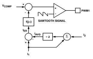
FIGURE 5. CHANNEL-1 PWM FUNCTION AND CURRENT-BALANCE ADJUSTMENT
