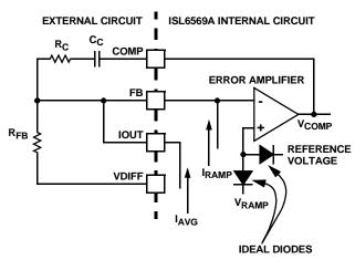
FIGURE 9. RAMP CURRENT AND VOLTAGE FOR REGULATING SOFT-START SLOPE AND DURATION
