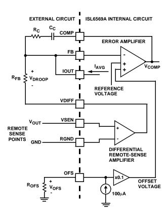
FIGURE 6. OUTPUT-VOLTAGE AND LOAD-LINE REGULATION
