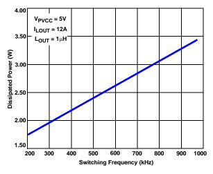
FIGURE 8. ISL6571 POWER DISSIPATION vs FREQUENCY AT 12A
