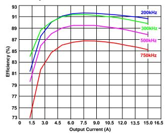
FIGURE 10. ISL6571 EFFICIENCY at 200kHz, 300kHz, 500kHz, 750kHz
