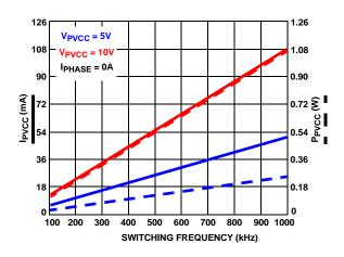
FIGURE 6. BIAS SUPPLY CURRENT/POWER vs FREQUENCY
