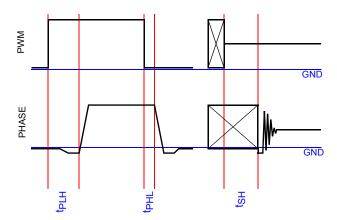
FIGURE 11. PHASE RESPONSE TO PWM INPUT
