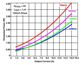
FIGURE 9. ISL6571 POWER DISSIPATION vs CURRENT at 200kHz, 300kHz, 500kHz, 750kHz
