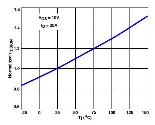
FIGURE 7. LOWER MOSFET ON RESISTANCE vs TEMPERATURE
