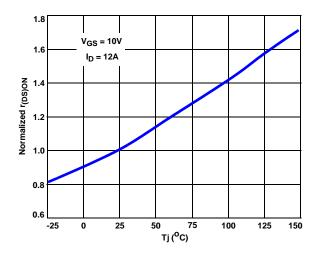
FIGURE 5. UPPER MOSFET ON RESISTANCE vs TEMPERATURE
