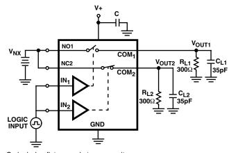
C<sub>L</sub> includes fixture and stray capacitance.
