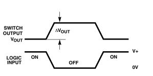
$Q = \Delta V_{OUT} \times C_{L}$
