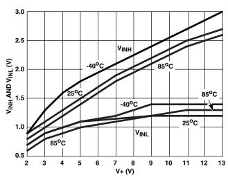
FIGURE 12. DIGITAL SWITCHING POINT vs SUPPLY VOLTAGE
