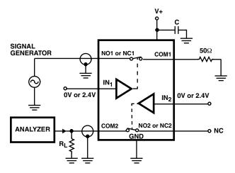
FIGURE 6. CROSSTALK TEST CIRCUIT
