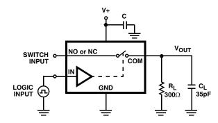
$\ensuremath{\text{C}_{\text{L}}}$  includes fixture and stray capacitance.
