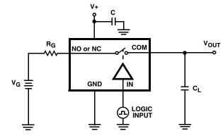
FIGURE 2A. MEASUREMENT POINTS
