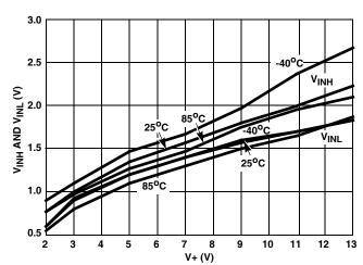
FIGURE 10. DIGITAL SWITCHING POINT vs SUPPLY VOLTAGE
