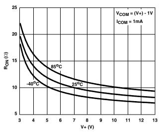
FIGURE 7. ON RESISTANCE vs SUPPLY VOLTAGE
