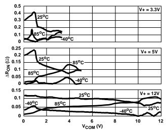
FIGURE 11. RON MATCH vs SWITCH VOLTAGE
