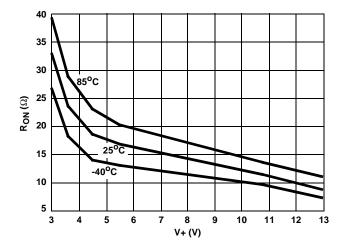
FIGURE 9. ON RESISTANCE vs SUPPLY VOLTAGE
