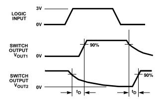
FIGURE 3A. MEASUREMENT POINTS (ISL84543 ONLY)
