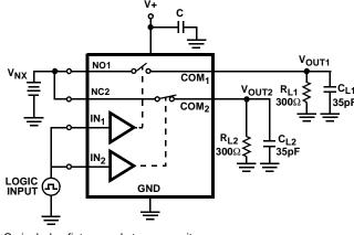
C<sub>L</sub> includes fixture and stray capacitance.
