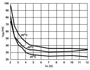
FIGURE 13. TURN - ON TIME vs SUPPLY VOLTAGE
