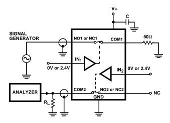
FIGURE 6. CROSSTALK TEST CIRCUIT
