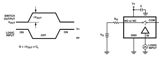
FIGURE 2A. MEASUREMENT POINTS
