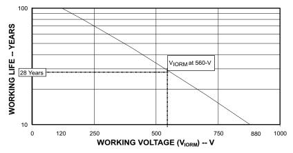
Figure 10. Time-Dependant Dielectric Breakdown Testing Results
