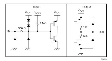
Figure 7. Device I/O Schematics
