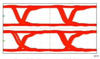
Figure 15. Eye Diagram at 200 MBPS, 5-V V<sub>CC</sub>, 125°C
