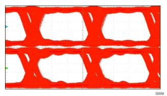
Figure 14. Eye Diagram at 250 MBPS, 5-V V<sub>CC</sub>, Typical
