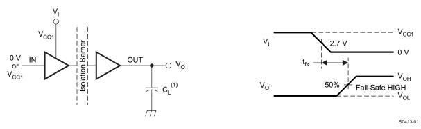
(1)  $C_L = 15 \text{ pF}$  and includes instrumentation and fixture capacitance within  $\pm 20\%$ .
