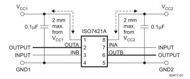
Figure 6. Typical ISO7421A Application Circuit
