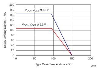
Figure 5.  $\theta_{JC}$  Thermal Derating Curve per IEC 60747-5-2
