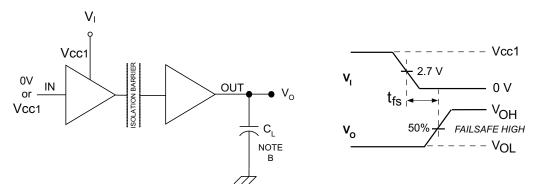
A.  $C_L = 15$  pF and includes instrumentation and fixture capacitance within  $\pm 20\%$ .
