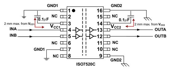
Figure 5. Typical ISO7520C Application Circuit
