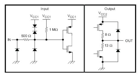
Figure 6. I/O Schematic
