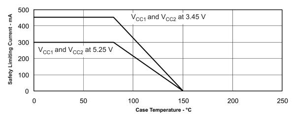
Figure 4. DW-16 Theta-JC Thermal Derating Curve per IEC 60747-5-2
