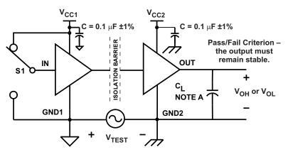
A.  $C_L = 15 \text{ pF}$  and includes instrumentation and fixture capacitance within ±20%.
