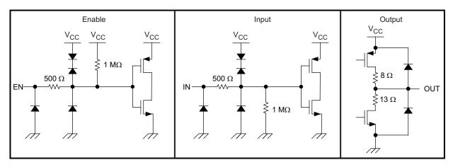
Figure 7. Device I/O Schematics
