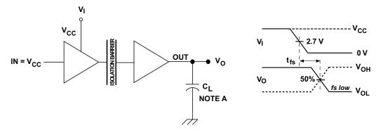
A.  $C_L = 15 \text{ pF}$  and includes instrumentation and fixture capacitance within ±20%.
