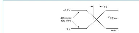
Fig 18. Receiver SE0 width tolerance.
