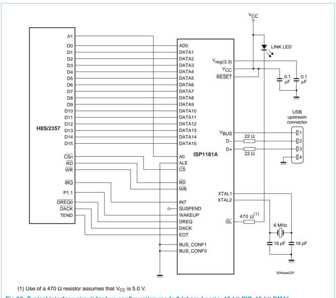
Fig 32. Typical interface circuit for bus configuration mode 0 (shared ports: 16-bit PIO, 16-bit DMA).
