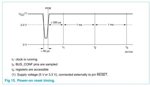
A hardware reset disables all USB endpoints and clears all ECRs, except for the control endpoint which is fixed and always enabled. Section 9.3 explains how to (re-) initialize the endpoints.
