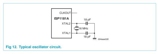
The 6 MHz oscillator frequency is multiplied to 48 MHz by an internal PLL. This frequency is used to generate a programmable clock output signal at pin CLKOUT, ranging from 3 to 48 MHz.
