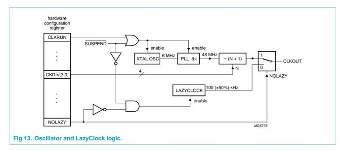
When ISP1181A enters 'suspend' state (by setting and clearing bit GOSUSP in the Mode Register), outputs SUSPEND and CLKOUT change state after approximately 2 ms delay. When NOLAZY = 0, the clock signal on output CLKOUT does not stop, but changes to the  $100 \pm 50\%$  kHz LazyClock frequency.
