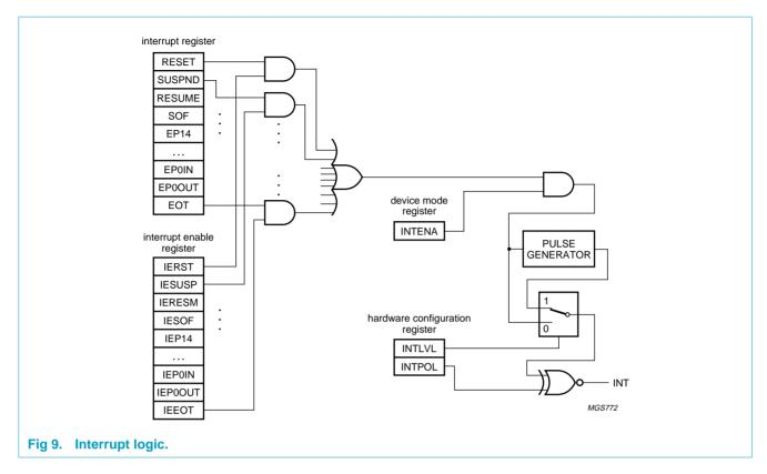
Bits RESET, RESUME, EOT and SOF are cleared upon reading the Interrupt Register. The endpoint bits (EP0OUT to EP14) are cleared by reading the associated Endpoint Status Register.
