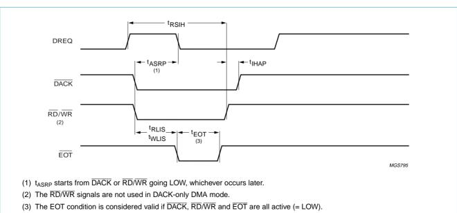
Fig 29. EOT timing in single-cycle DMA mode.
