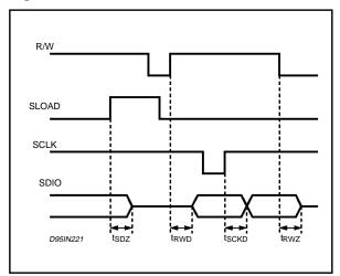
L6239 is deselected by bring SLOAD high, the serial port stops writing and assumes a tri-state condition after time t<sub>STZ</sub>.
