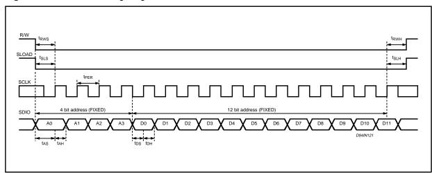
Figure 1: Serial Write Timing Diagram
