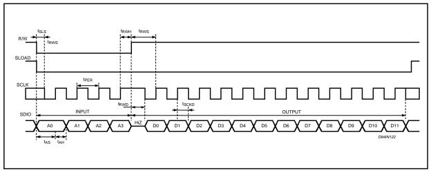
The write cycle has a fixed address and data length. Four bits of address and 12 bits of data must be clocked in to allow the data to be loaded into the desired register.
