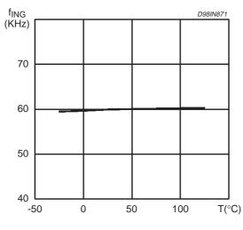
Figure 6. f<sub>PRE</sub> vs. temperature.
