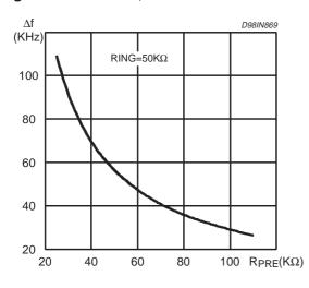
Figure 4.  $\Delta f$  vs. R<sub>PRE</sub>, with R<sub>ING</sub> = 100k $\Omega$
