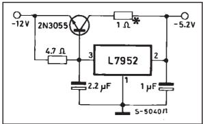
Optional dropping resistor to reduce the power dissipated in the boost transistor.
