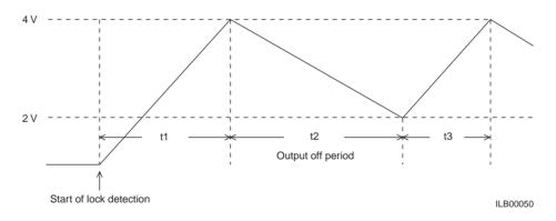
The following formula gives the time, t1, from the point the motor speed is locked until the output is turned off.  $t1[s] = C [\mu F] \times 4 [V] / 1 [\mu A]$
