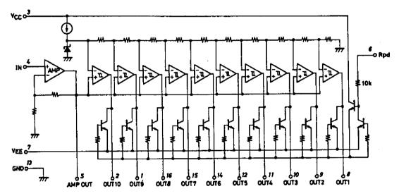
Sample Application Circuit: Signal Meter
