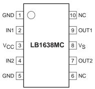
Note: both ground pins must be grounded.
