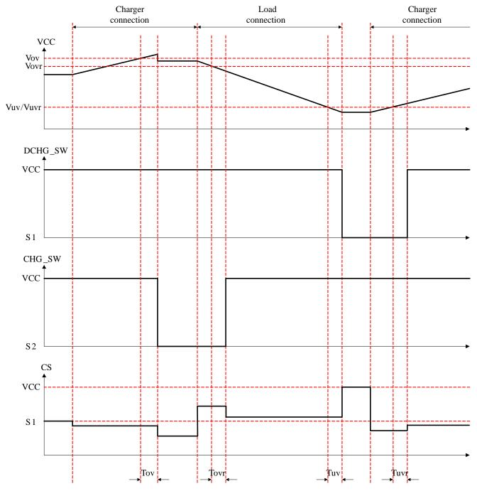
Figure 6. Over-charged detection/release, Over-discharge detection/release (Connect charger)
