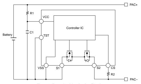
Figure 1. Example of Application Circuit
