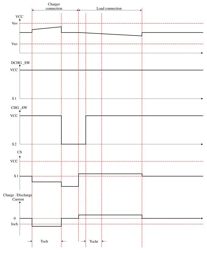
Figure 9. Charge Over-current Detection
