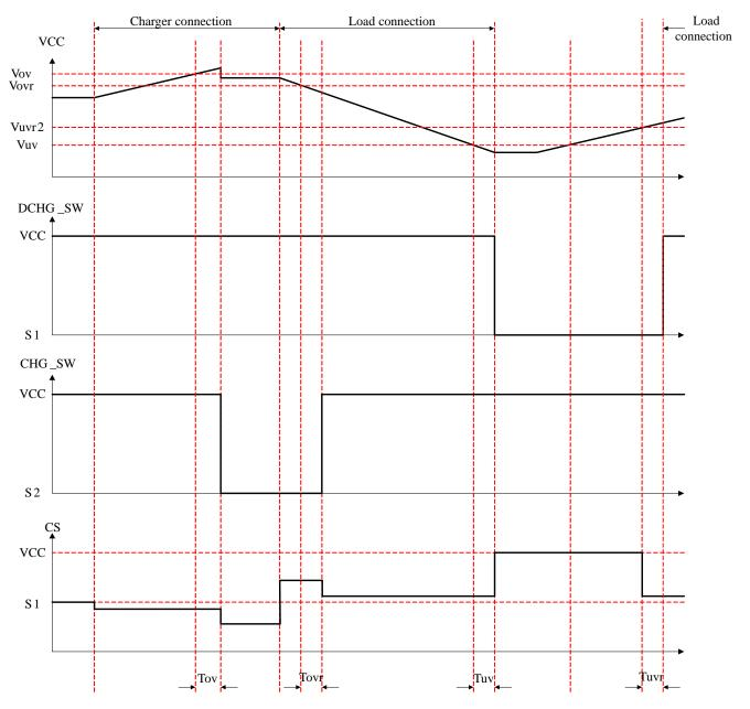
Figure 7. Over-charge detection/release, Over-discharged detection/release (Non-connect charger)
