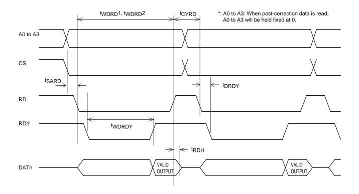
• Post-Correction Data Read Timing (DMA)
