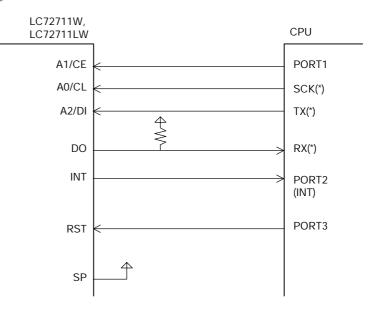
\* SCK, TX, and RX are the CPU serial interface channel. Normally, I/O port pins may be used for these lines. \* The resistance of the DO pin pull-up resistor must be selected according to the transfer clock speed.
