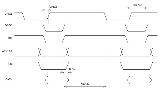
\*: A0 to A3: When post-correction data is read, A0 to A3 will be held fixed at 0.
