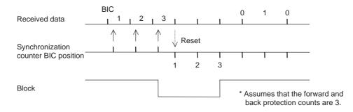
Figure 1 Block Synchronization Protection Operation (Forward  $\rightarrow$  Back  $\rightarrow$  Forward)
