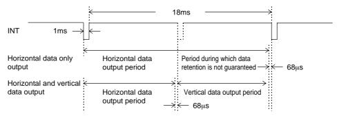
Figure 2 External Interface - Basic Timing
