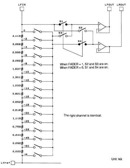
When data specifying a  $-\infty$  attenuation in the 2 dB step main volume is issued, S1 and S2 will open and at the same time, S3 and S4 will turn on.
