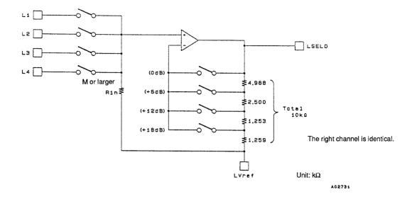
10 dB Step Volume Equivalent Circuit
