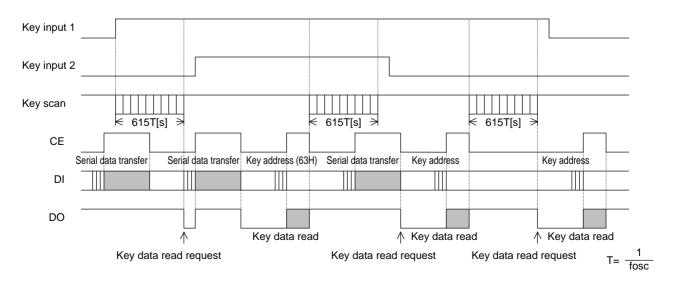
Example: When control data "KP1 and KP2 = 0, KC1 to KC5 = 0, KC6 = 1" are executed. (i.e.key scanning with only KS6 high.)
