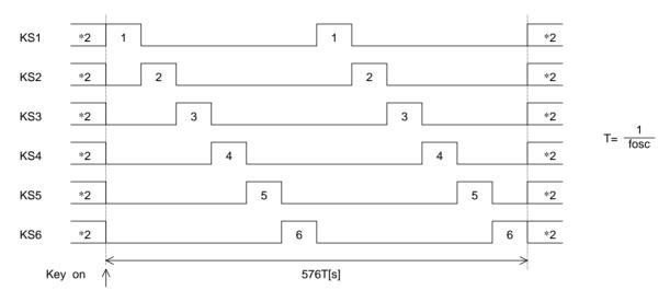
\*2. Not that the high/low states of these pins are determined by the control data, and that key scan output signals are not output from pins that are set to low .
