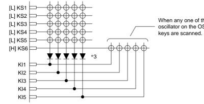
When any one of these keys is pressed, the oscillator on the OSC pin is started and the keys are scanned.
