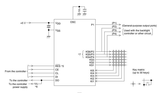
Note: \*5. When the power is first applied, it must be initialized by  $\overline{RES} = "L"$ .
