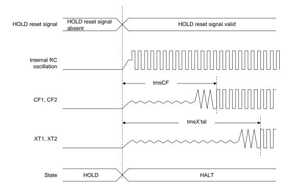
HOLD Reset Signal and Oscillation Stabilization Time
