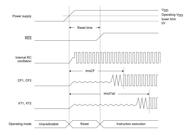
Reset Time and Oscillation Stabilization Time
