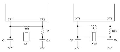
Figure 1 CF Oscillator Circuit
