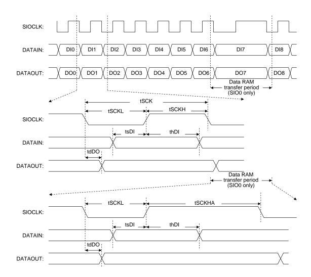
Figure 6 Serial I/O Waveforms
