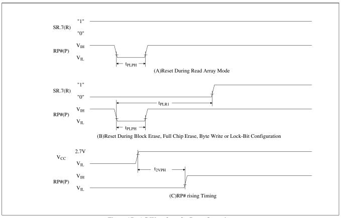
Figure 17. AC Waveform for Reset Operation
