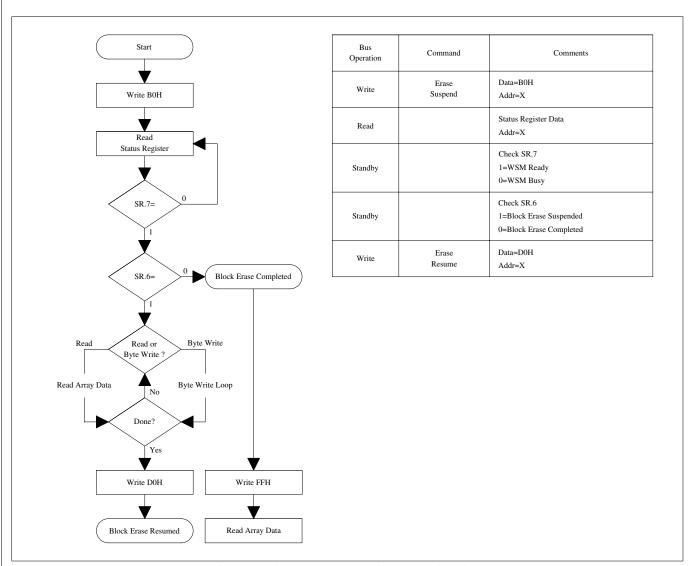
Figure 8. Block Erase Suspend/Resume Flowchart
