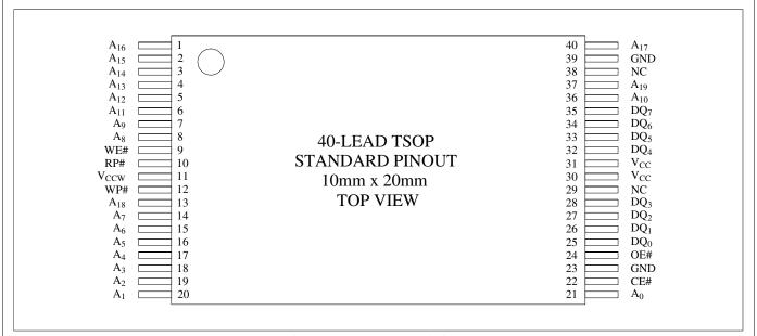
Figure 2. TSOP 40-Lead Pinout
