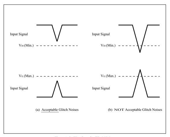
Figure A-2. Waveform for Glitch Noises
