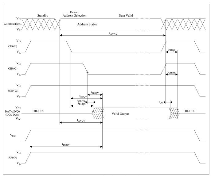
Figure 14. AC Waveform for Read Operations
