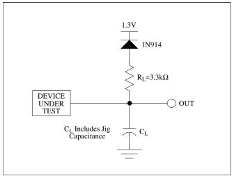
Figure 13. Transient Equivalent Testing Load Circuit
