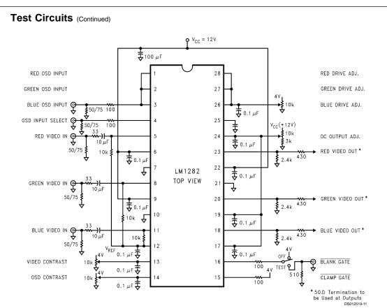
FIGURE 6. LM1282 OSD Video Preamp AC Test Circuit
