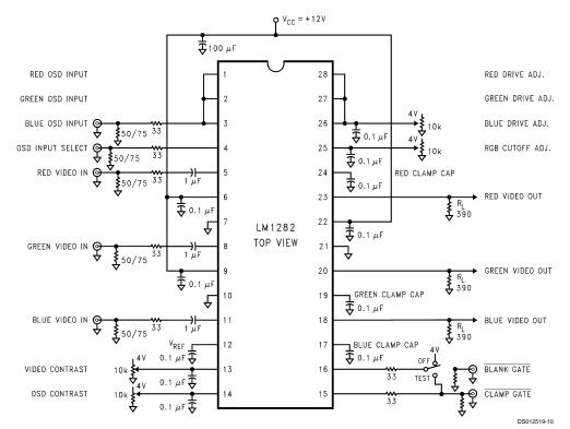
FIGURE 5. LM1282 OSD Video Preamp DC Test Circuit
