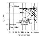
Figure 4. -3 dB Bandwidth vs Frequency and Control Signal
