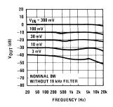
Figure 3. Output vs Frequency
