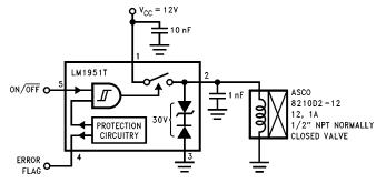
FIGURE 1. Solenoid Actuated Valve
