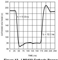
Figure 12. LM2422 Cathode Response
