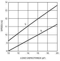
Figure 7. Speed vs Load Capacitance
