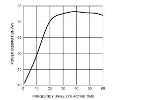
Figure 10. Power Dissipation vs Frequency
