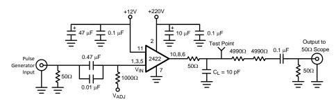
Note: 10 pF load includes parasitic capacitance.
