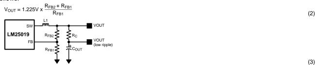
This regulator regulates the output voltage based on ripple voltage at the feedback input, requiring a minimum amount of ESR for the output capacitor (C<sub>OUT</sub>). A minimum of 25mV of ripple voltage at the feedback pin (FB) is required for the LM25019. In cases where the capacitor ESR is too small, additional series resistance may be required (R<sub>C</sub> in Figure 13 Low Ripple Output Configuration).
