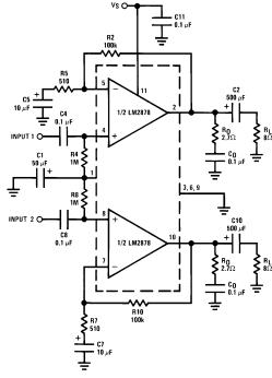
FIGURE 3. Stereo Amplifier with  $A_V = 200$
