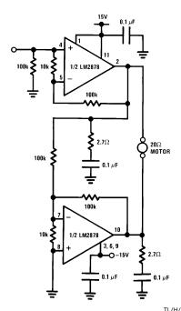
FIGURE 4. LM2878 Servo Amplifier in Bridge Configuration
