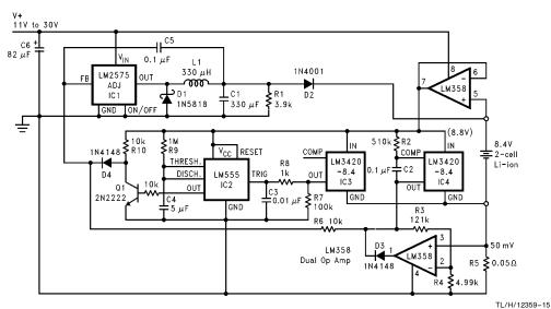
FIGURE 10. (Fast) Pulsed Constant Current 2-Cell Charger
