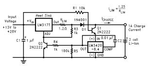
FIGURE 5. Constant Current/Constant Voltage Li-lon Battery Charger
