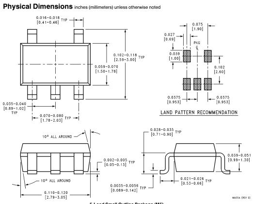
5-Lead Small Outline Package (M5) For Ordering Information See Figure 1 In This Data Sheet NS Package Number MA05A
