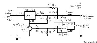
Typical Constant Current/Constant Voltage Li-Ion Battery Charger
