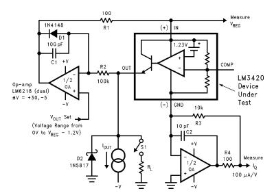
FIGURE 2. LM3420 Test Circuit
