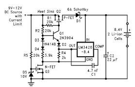
FIGURE 11. MOSFET Low Dropout Charger
