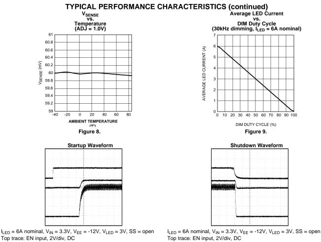
Middle trace:  $V_{EE}$  input current, 2A/div, DC Bottom trace:  $I_{LED}$ , 2A/div, DC T = 100µs/div
