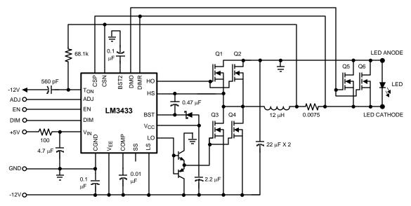
Figure 14. 2A to 14A Output Application Circuit
