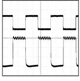
$$\begin{split} I_{LED} &= 6A \text{ nominal, } V_{IN} = 3.3V, V_{EE} = -12V\\ \text{Top trace: DIM input, } 2V/div, DC\\ \text{Bottom trace: } I_{LED}, 2A/div, DC\\ T &= 10 \mu s/div \end{split}$$
