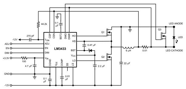
Figure 13. 2A to 6A Output Application Circuit
