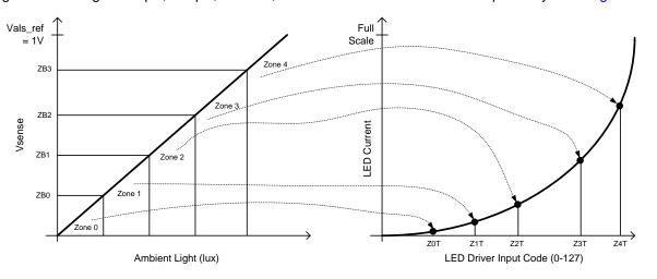
Figure 41. ALS Zone to LED Brightness Mapping
