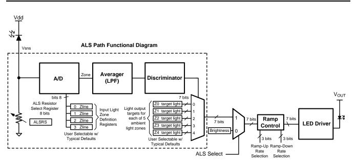
Figure 40. Ambient Light Sensor Functional Block Diagram
