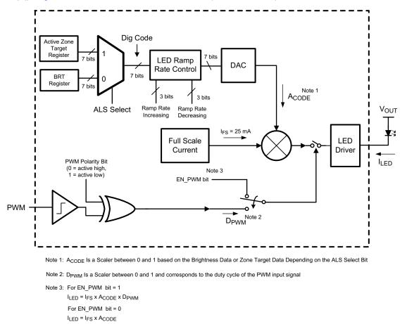
Figure 46. Current Control Block Diagram
