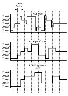
Figure 44. Ambient Light Input to Backlight Mapping
