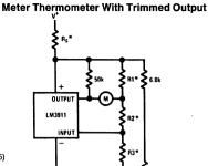
\*Selected as for meter thermometer except To should be 5°K more than desired and  $I_{\Omega} = 100 \ \mu A$ †Calibrates To
