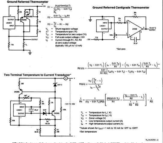
\*\* The 0.01 in the above and following equations is in units of V/°K or V/°C, and is a result of the basic 0.01V/°K sensitivity of the transducer
