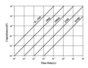
Figure 2. Resistance and Capacitance vs. Time delay(t<sub>d</sub>)
