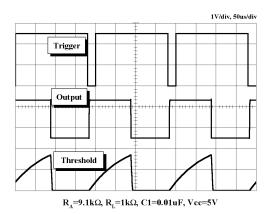
Figure 3. Waveforms of Monostable Operation
