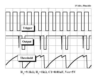
Figure 4. Waveforms of Monostable Operation (abnormal)
