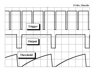
$R_A=9.1k\Omega$ ,  $R_T=1k\Omega$ , C1=0.01uF, Vcc=5V
