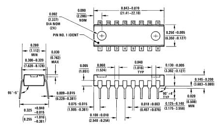
16-Lead Molded Dual-In-Line Package (N) Order Number LM6313N NS Package Number N16A
