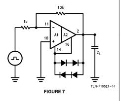
In photo 1,  $C_L$  is 1000 pF. The LM6313 is slewing at 250 V/ $\mu s$ , from -5 V to +5 V. The slew rate is 450 V/ $\mu s$ from +5V to -5V. This requires the op amp to deliver
