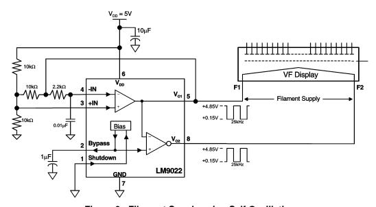
Figure 9. Filament Supply using Self Oscillation
