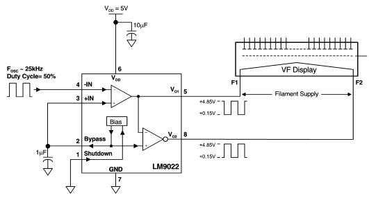
Figure 8. Filament Supply using External Oscillator
