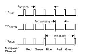
Figure 38: 3 Channel Line Rate TR Pulse Timing
