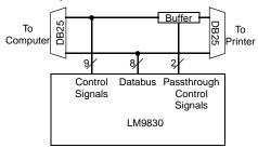
Figure 50: Printer Passthrough Overview
