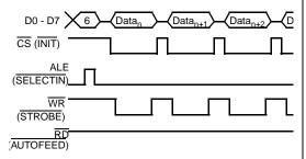
Figure 58: Writing to the Configuration Register (μP)
