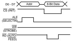
Figure 57: Reading from the Configuration Register (µP mode, except DataPort)
