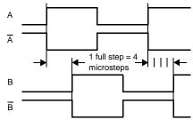
Figure 16: Stepper Motor Waveform - Full Stepping
