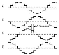
Figure 18: Bipolar Microstepping Waveform
