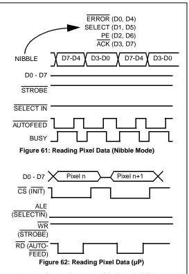
Image data can flow as fast as possible from the LM9830 to the host, but can be interrupted at any time (by latching a different address) to read the LM9830's status registers, abort the scan, etc.
