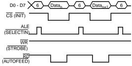
Figure 59: Reading Gain and Offset Coefficients through the DataPort (µP mode)
