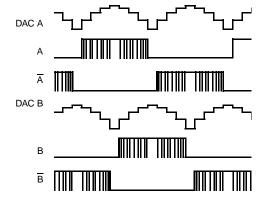
Figure 19: Stepper Motor Waveform - LM9830 Signals
