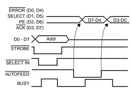
Figure 55: Reading from the Configuration Register (Nibble Mode)
