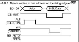
Figure 56: Writing to the Configuration Register (µP)
