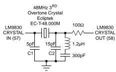
Figure 63: Crystal Oscillator Circuit
