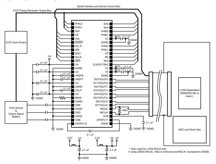
Figure 3. Typical Application Diagram
