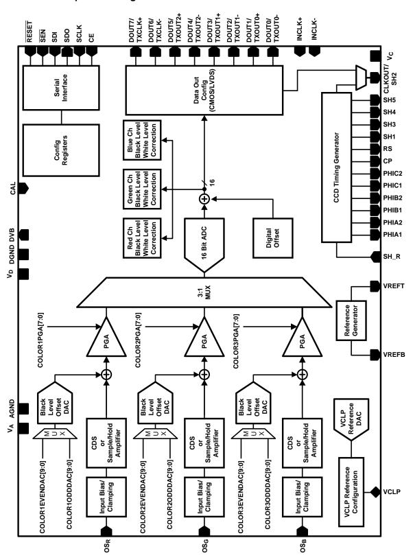
Figure 1. Chip Block Diagram
