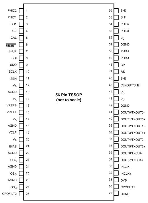
Figure 2. TSSOP Package See Package Number DGG0056A
