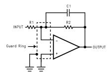
Figure 8. (a) Inverting Amplifier
