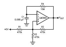
Figure 17. 1 Hz Square-Wave Oscillator
