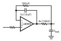
Figure 5. Rx, Cx Improve Capacitive Load Tolerance
