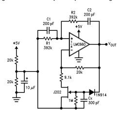
Figure 16. Sine-Wave Oscillator
