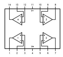
Figure 1. 14-Pin DIP/SO
