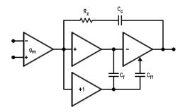
Figure 2. LMC660EP Circuit Topology (Each Amplifier)
