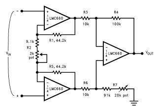
Figure 15. Instrumentation Amplifier
