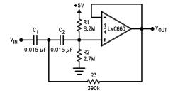
$$\begin{split} &f_c = 10 \text{ Hz} \\ &d = 0.895 \\ &Gain = 1 \\ &2 \text{ dB passband ripple} \end{split}$$
