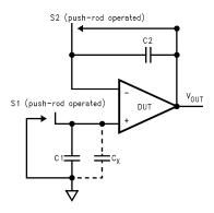
Figure 13. Simple Input Bias Current Test Circuit
