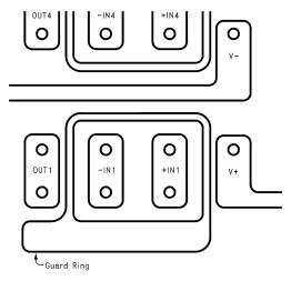
Figure 7. Example, using the LMC660AIMEP, of Guard Ring in P.C. Board Layout
