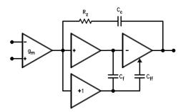
Figure 3. LMC660EP Circuit Topology (Each Amplifier)
