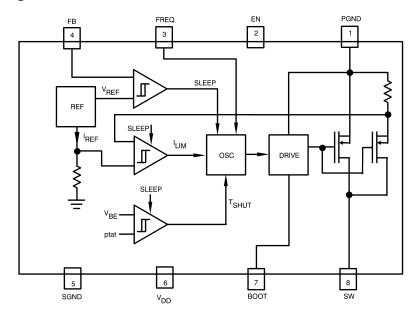
Figure 4. Block Diagram
