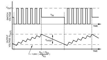
Figure 5. Typical Step-Up Regulator Waveforms
