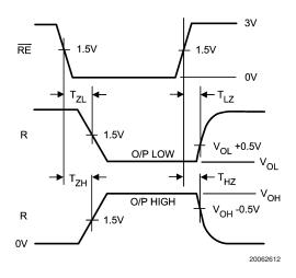
FIGURE 10. Receiver Enable / Disable Time
