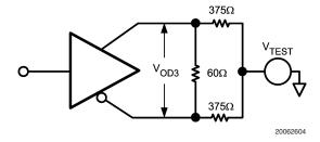
FIGURE 2. Test Circuit for  $V_{\text{OD3}}$
