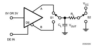
FIGURE 4. Test Circuit for Driver Enable / Disable
