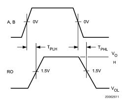
FIGURE 9. Receiver Propagation Delay
