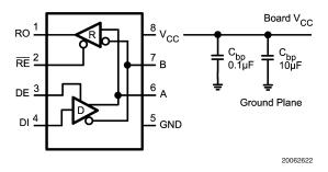
FIGURE 11. Placement of by-pass Capacitors, C<sub>bp</sub>
