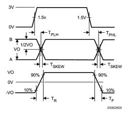
FIGURE 7. Driver Propagation Delay, Rise / Fall Time
