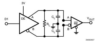
FIGURE 5. Test Circuit for Receiver Propagation Delay
