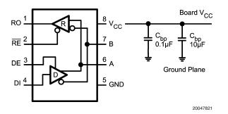
FIGURE 9. Placement of by-pass Capacitors, C<sub>bp</sub>
