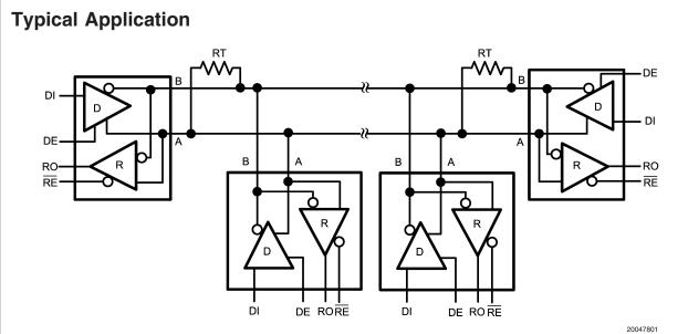
A Typical multipoint application is shown in the above figure. Terminating resistors, RT, are typically required but only located at the two ends of the cable. Pull up and pull down resistors maybe required at the end of the bus to provide failsafe biasing. The biasing resistors provide a bias to the cable when all drivers are in TRI-STATE, See National Application Note, AN-847 for further information. MS75ALS176A Differential Bus Transceivers
