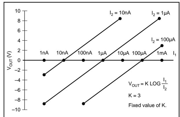
FIGURE 3. Transfer Function with Varying  $I_2$  and  $I_1$ .
