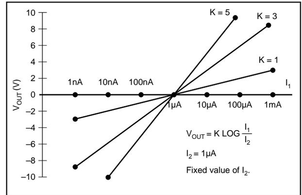
FIGURE 2. Transfer Function with Varying  $K$  and  $I_1$ .
