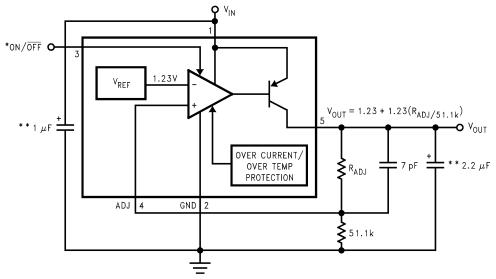
\*ON/ $\overline{\text{OFF}}$  INPUT MUST BE ACTIVELY TERMINATED. TIE TO V<sub>IN</sub> IF THIS FUNCTION IS NOT TO BE USED. \*\*MINIMUM CAPACITANCE IS SHOWN TO ENSURE STABILITY OVER FULL LOAD CURRENT RANGE (SEE APPLICATION HINTS).
