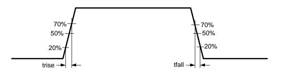
Figure 4. Output Transition Time (A and B Side)
