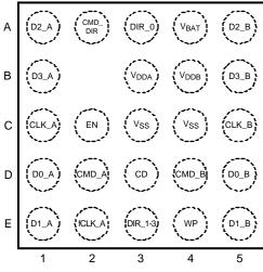
Figure 1. Bump Underneath (Top View) 24 Bump DSBGA Package See Package Number YFR0024AAA
