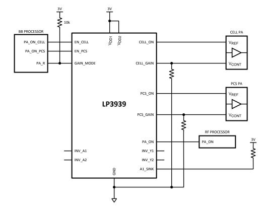
NOTE: This application circuit shows the connection interface to a typical Skyworks PA. Connections to other PA vendors may vary slightly.
