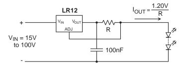
Figure 3: High Voltage Adjustable Constant Current Source
