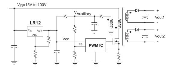
Figure 2: SMPS Start-Up Circuit
