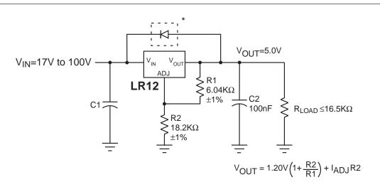
Figure 1: High Input Voltage, 5.0V Output Linear Regulator
