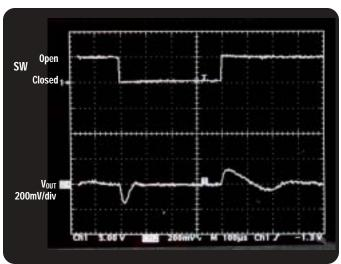
Load Transient Response, Load=509 $\Omega$
