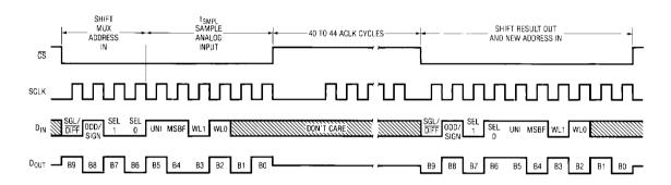
Figure 3. CS High During Conversion
