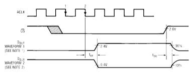
NOTE 1: WAVEFORM 1 IS FOR AN OUTPUT WITH INTERNAL CONDITIONS SUCH THAT THE CUTPUT IS HIGH UNLESS DISABLED BY THE OUTPUT CONTROL.
