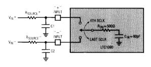
Figure 9. Analog Input Equivalent Circuit
