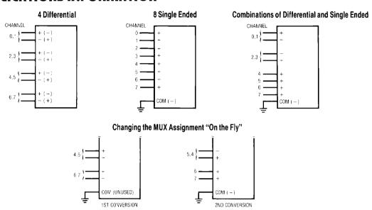
Figure 1. Examples of Multiplexer Options on the LTC1090
