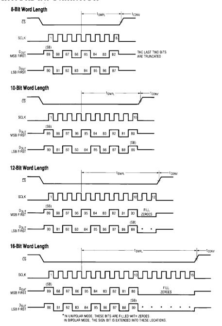
Figure 2. Data Output (D<sub>OUT</sub>) Timing with Different Word Lengths
