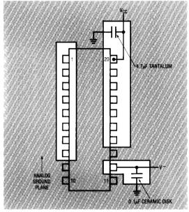
Figure 6. Example Ground Plane for the LTC1090
