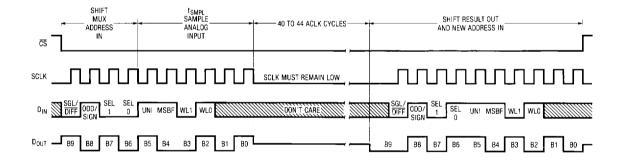
Figure 4. CS Low During Conversion
