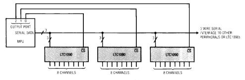
Figure 5. Several LTC1090s Sharing One 3 Wire Serial Interface
