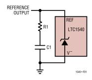
Figure 1. Damping the Reference Output
