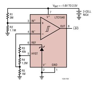
Figure 9. Low-Battery Detect Works Down to 1.6V
