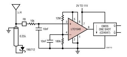
Figure 10. Nanopower Field Detector
