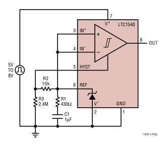
Figure 3a. Power Supply Transient Test Circuit
