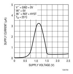
Figure 4. Supply Current vs Supply Voltage
