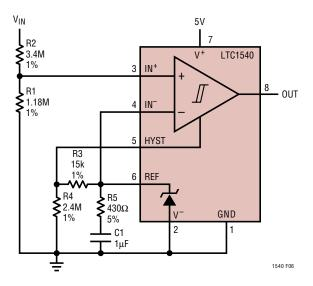
Figure 6. Glitch-Free Level Detector with Hysteresis
