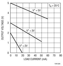
Comparator Output Voltage (Low) vs Load Current
