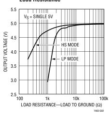
**Output Voltage Swing High vs Load Resistance**
