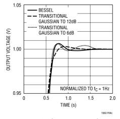
Figure 6c. Step Response—Settling
