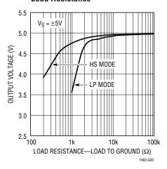
**Output Voltage Swing Low vs** Load Resistance
