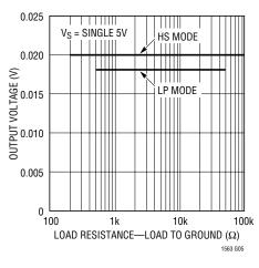
**Output Voltage Swing Low vs Load Resistance**
