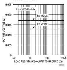
**Output Voltage Swing Low vs Load Resistance**
