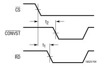
Figure 4.  $\overline{\text{CS}}$  to  $\overline{\text{CONVST}}$  Setup Timing
