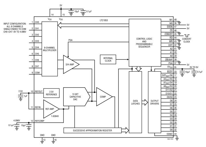
LTC1853 Configured for 8-Channel, Unipolar, Single-Ended Operation
