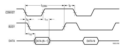
Figure 9. ROM Mode Timing,  $\overline{CS} = 0$
