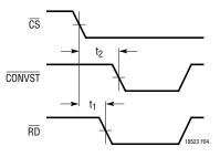
Figure 3. SHDN to CONVST Wake-Up Timing
